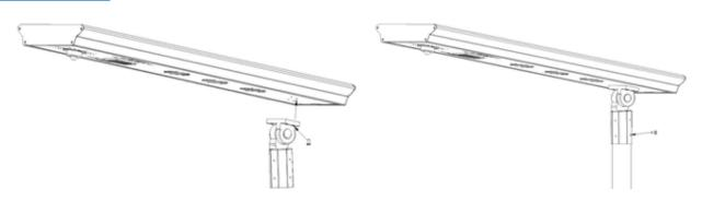
Use 4 screws each to fix the support on the lamp and fix the lamp on the pole.
